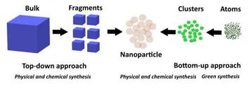
Figure 2. Nanoparticle's synthesis approaches [8]
