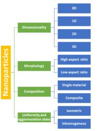
Figure 3. Nanoparticles' classification [8]
