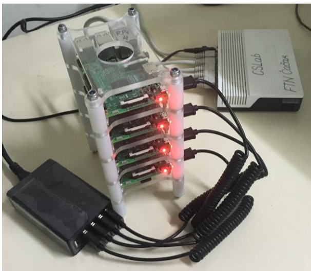
Figure 6. The appearance of the Raspberry Pi 3 cluster
