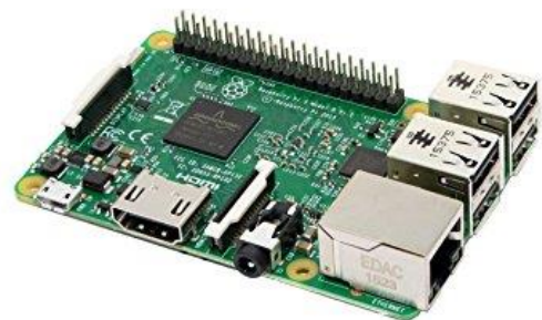
Figure 4. The appearance of Raspberry Pi 3 Model B
