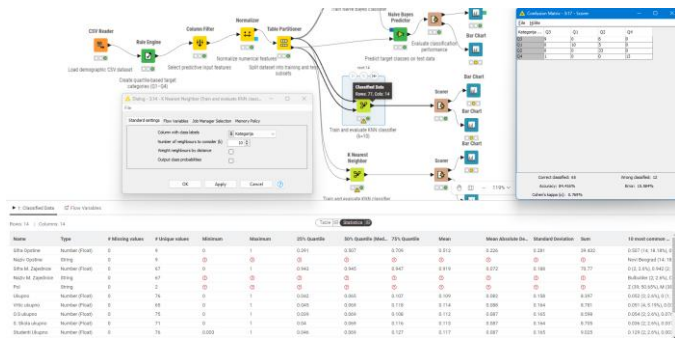
Figure 10. KNN ( k = 10 ) classification results in KNIME, including the confusion matrix, overall accuracy, and error statistics
