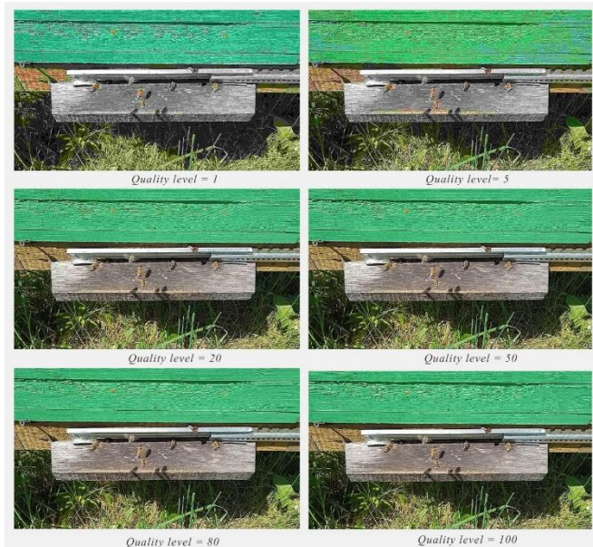
Figure 9. Comparison of compressed image versions at different quality levels (Q); lower Q values cause blocking artifacts and loss of sharpness, while higher values preserve better visual fidelity with reduced image size.
