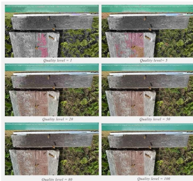
Figure 5. Comparison of compressed image versions at different quality levels (Q); lower Q values cause blocking artifacts and loss of sharpness, while higher values preserve better visual fidelity with reduced image size.
