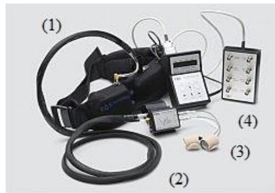
Figure 1. Portapres® system: (1) The waist belt-contains sections for the main unit (electronics and memory card, air pump and lithium battery - allows 60 hours of operation in transmissive mode) (2) Frontend Unit for Portapres® (double finger cuffs systems) (3) set of cuffs (large, medium and small) (4) output box (A/D converter) [10].
