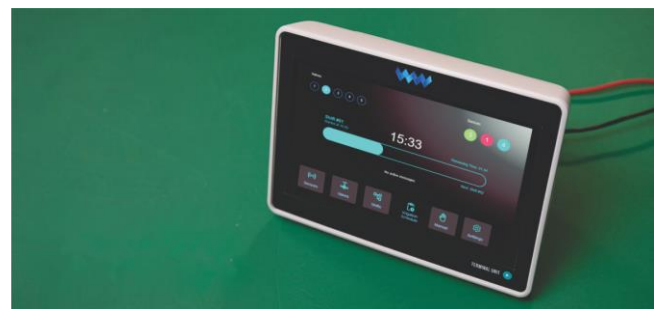
Figure 2. Realized prototype of terminal unit.
