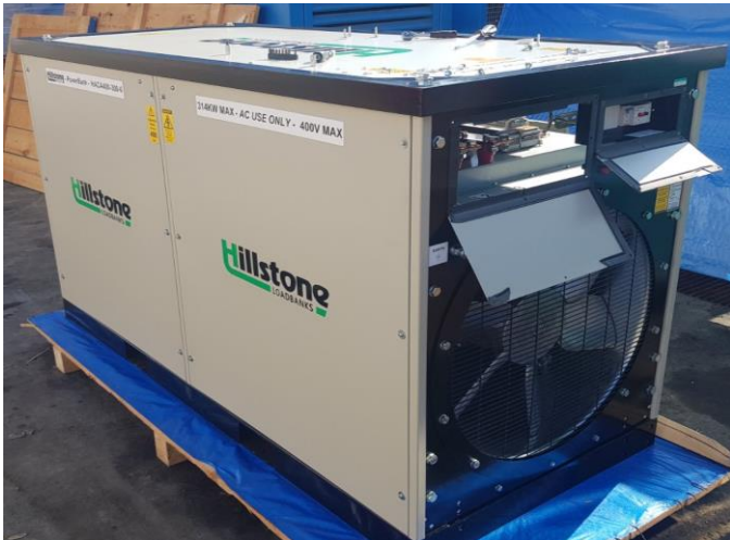
Figure 3. Hillstone load bank 3 phase AC, 400V, 319 kW
