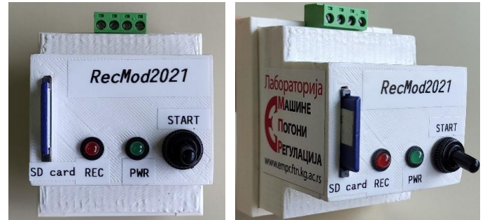
Figure 10. 3D model (top) and final look of the developed RecMod2021 device - ver. 1 (bottom)
